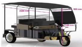
Figure 34. 3-D view and dimensions of the proposed e-rickshaw.
