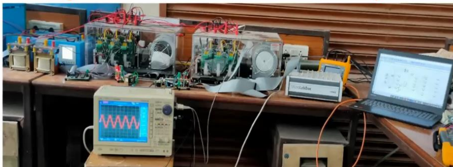
Fig. 22. Prototype of MMLI based grid connected solar PV system
