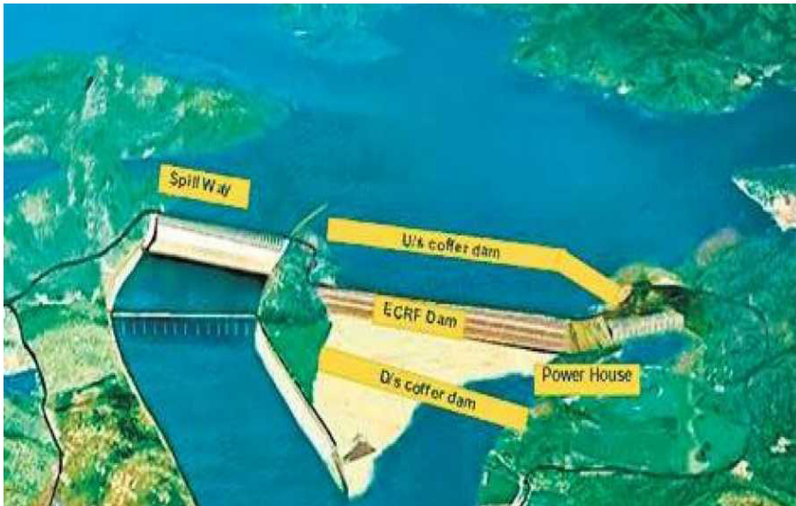
Photograph of Polavaram Irrigation Project – Andhra Pradesh, India as part of presentation
