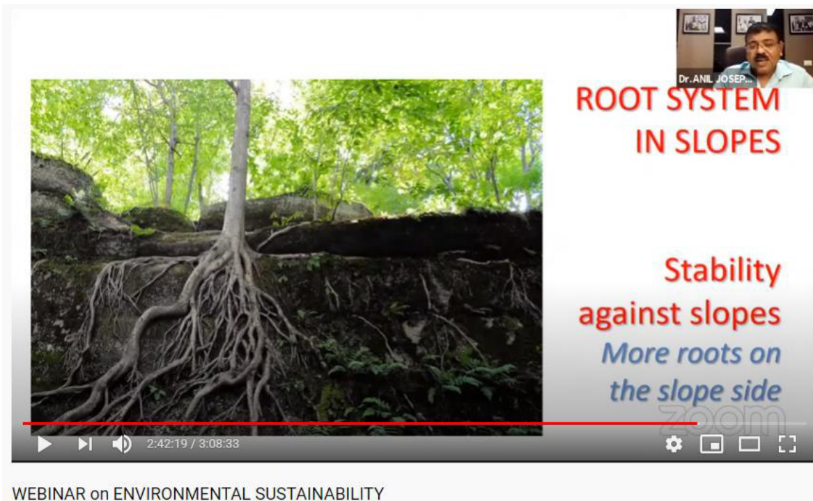
Figure 10: Root Systems Stabilizing the Slopes
