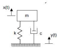
2. An analytical expression for the response of a damped single degree of freedom system to given initial displacement and velocity is given by
