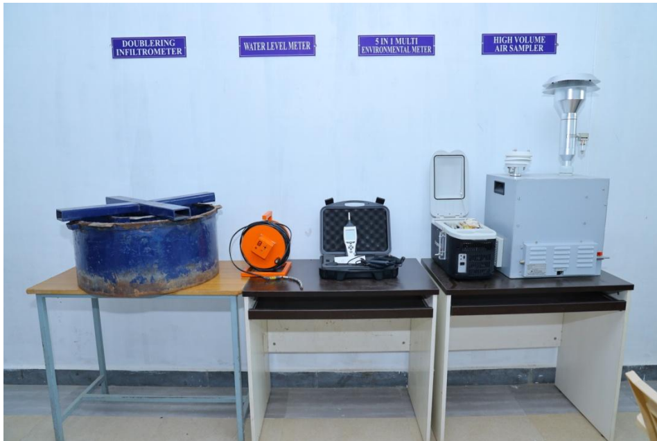
Double Ring Infiltrrometer, Water Level Indicator, 5 in 1 Multi Enviro-meter and Ambient Fine Dust Sampler
