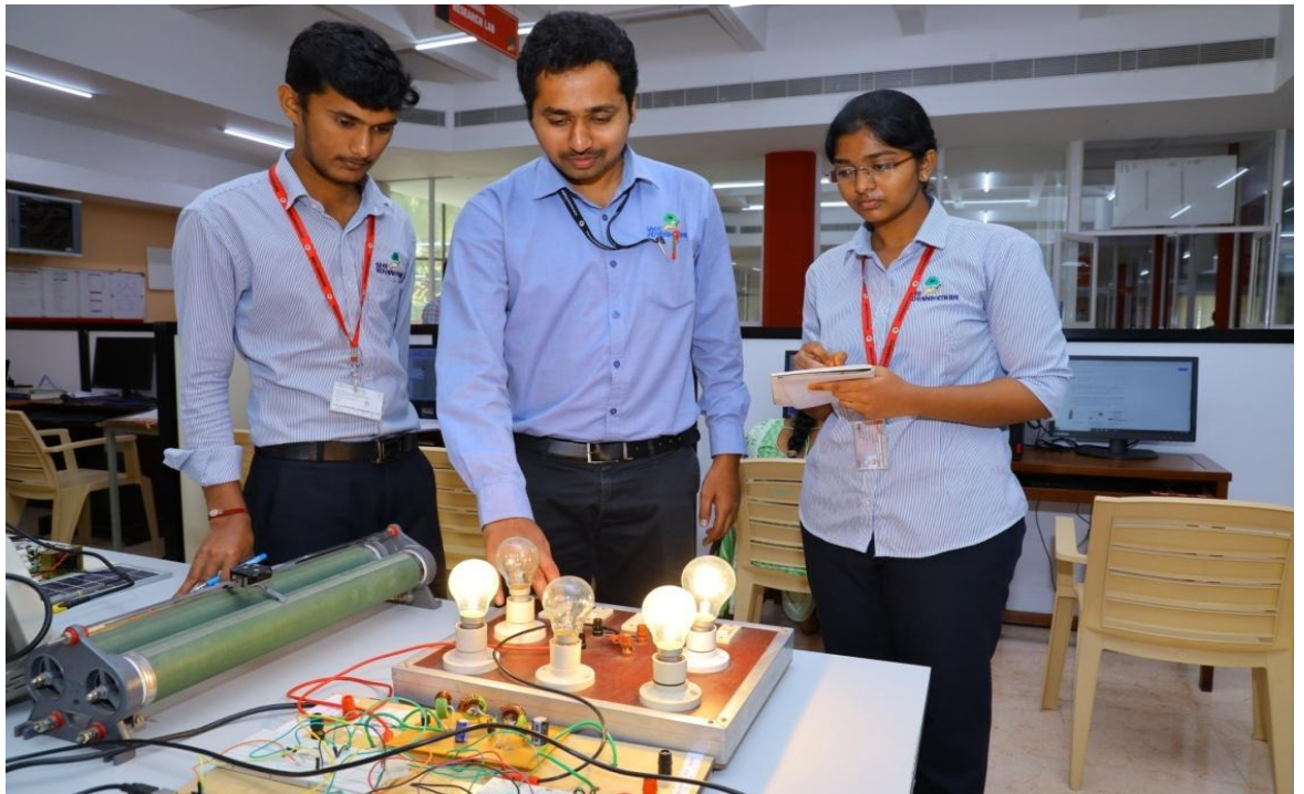
Single phase Inverter testing under loaded condition using lamps
