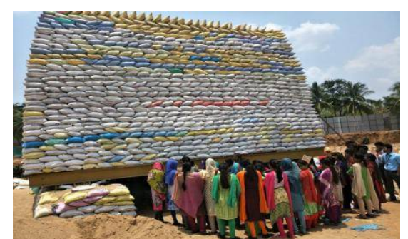
Dr. O. Eswara Reddy explaining the Procedure of Pile Load Test
