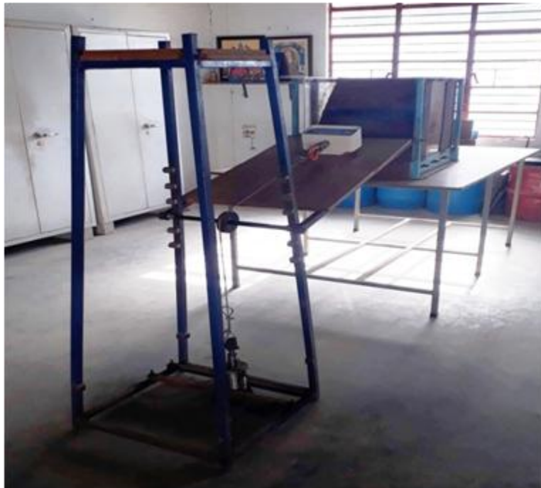
Experimental Setup for Pullout Tests on Geosynthetic Reinforced Soil Slopes
