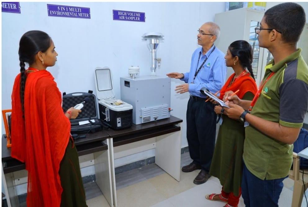
5 in 1 Multi Enviro-meter and Ambient Fine Dust Sampler
