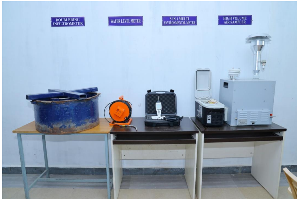
Double Ring Infiltrometer, Water Level Indicator, 5 in 1 Multi Enviro-meter and Ambient Fine Dust Sampler
