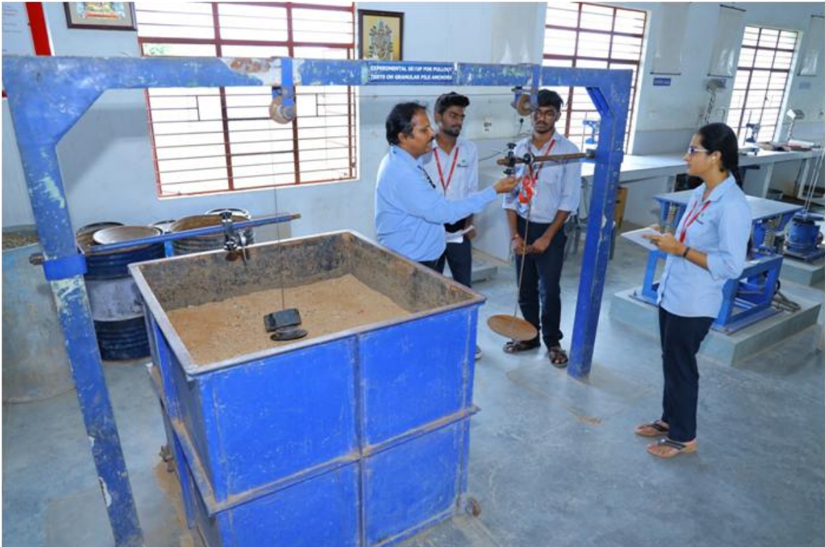
Experimental Setup for Pullout Tests on Granular Pile Anchors
