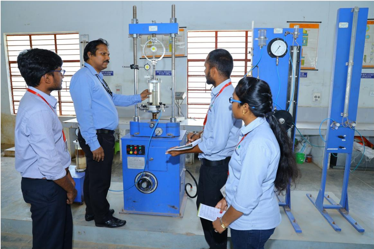
Triaxial Compression Testing Machine with Pore Pressure Measurement
