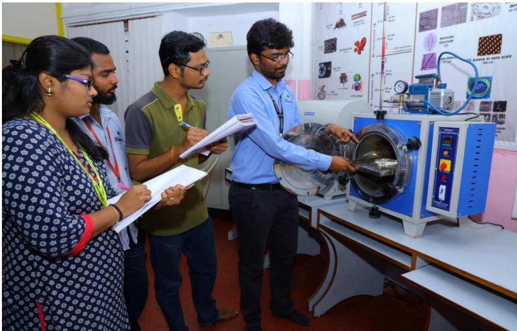
Vacuum Furnace for Annealing Purpose
