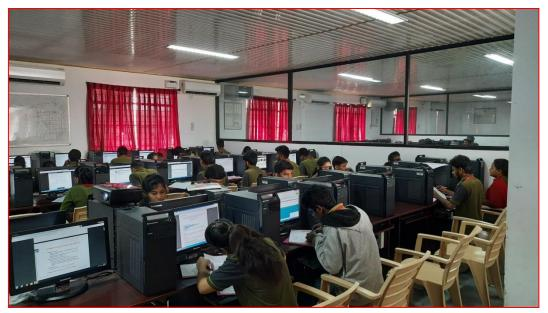
The **Advanced Programming Lab – I(Lab-B)** consists of **46** systems with Intel core i3 - 4150 @ 3.30 GHz Processors, 4<sup>th</sup> Generation, 8GB DDR3 RAM, 500 GB Hard disk, 18.5" LCD Lenovo Monitor (Lenovo Think Center) configuration in area of 75 Sq.M to conduct Database Management Systems, Object oriented Programming and Object Oriented Analysis and Design Laboratories.
